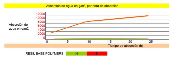
Absorption of water of a basic coating with, and another without polymeric dusts dispersables hidrófobos, probeta of cellular concrete
