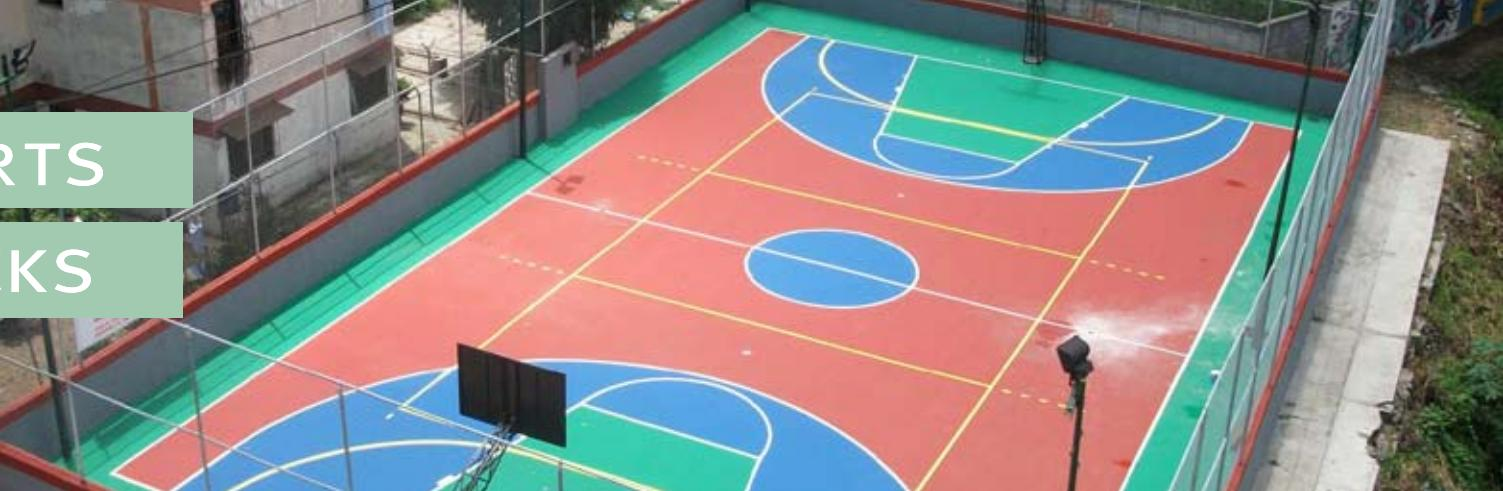
The good performance of polyurea against climatic change and the outdoors, as well as its anti-abrasion resistance, adherence and colouring possibility, makes this the ideal material for applying to multi-purpose sports tracks.
